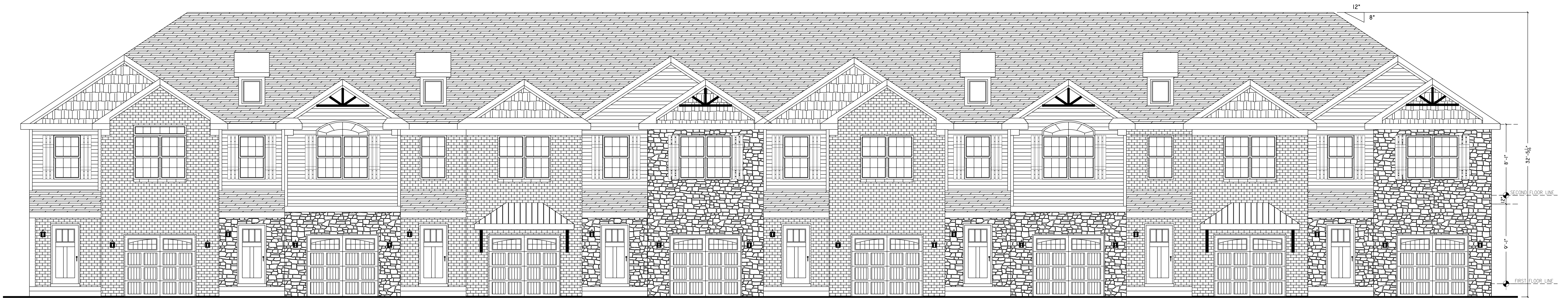
EIGHT PLEX FRONT ENTRY FRONT ELEVATION
