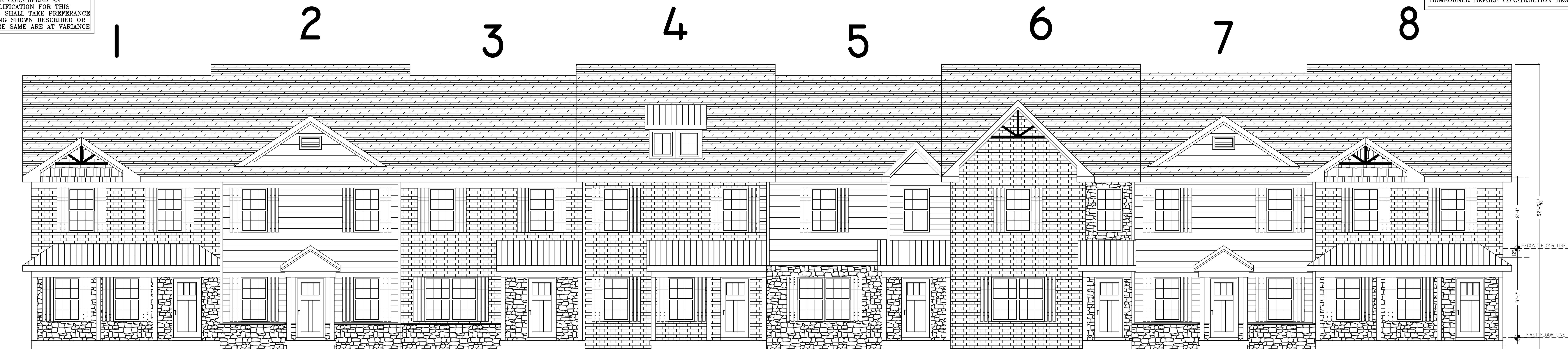
EIGHT PLEX REAR ENTRY FRONT ELEVATION
