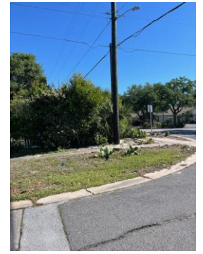
Obstructed Vision Triangle (Seaview and Beach looking north). Had to pull up into Pedestrian walkway to see
