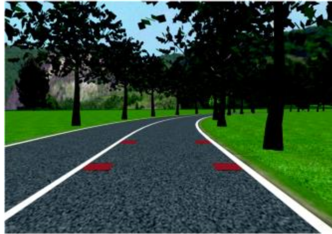
Red peripheral transverse bars
