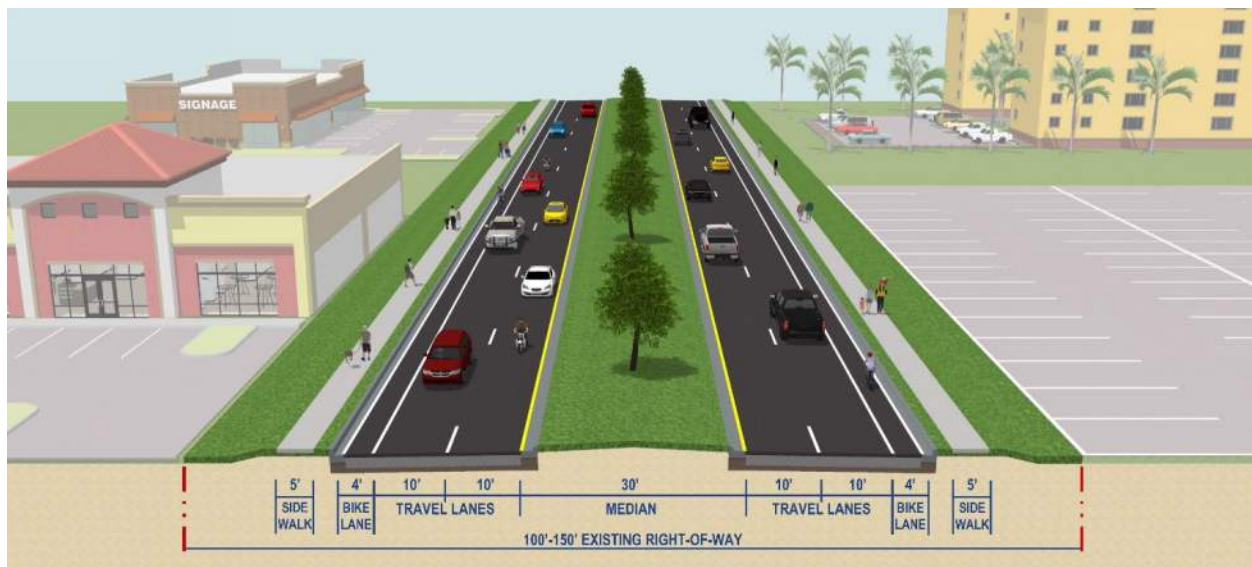
Figure 2.1.1: Existing Typical Section
